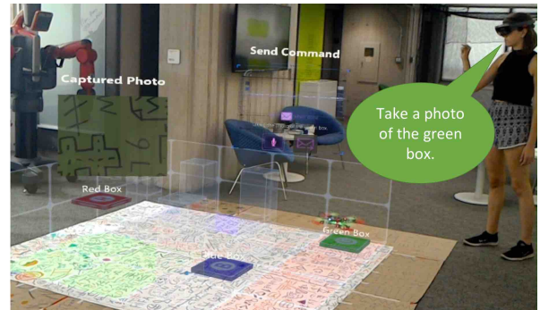
Fig. 1: An example of a task-oriented navigational command given to a drone through the MR interface with language. The scene is clear when displayed via the HoloLens.
