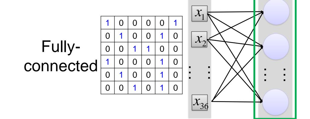
Conventional Fully Connected layers (FC layers)
