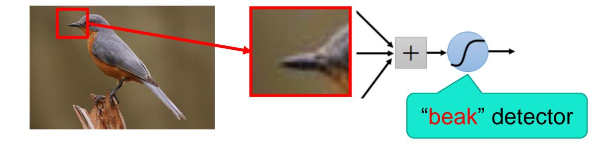
Same pattern appears in different places: They can be compressed! What about training a lot of such "small" detectors and each detector must "move around".
